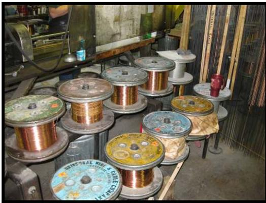
A bass string manufacturer (there are several highly-reputed shops to choose from depending upon the needs of your piano) must have a complete inventory of both the gauges of steel core strings and also the diameters of copper windings which are used to "load" the strings.
