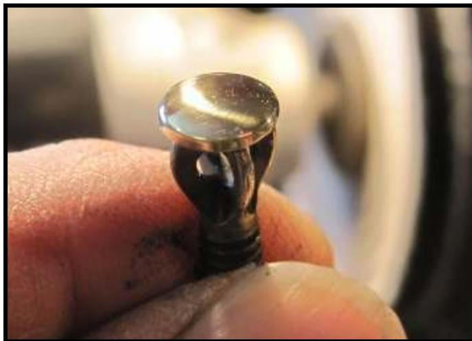
With the capstans of your piano polished as in the above photo, wear and tear on the corresponding felts will be at a minimum, and performance will be at a maximum.
