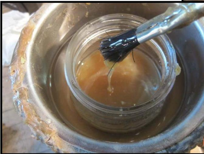
Depending on the circumstances, either a cold glue or a hot glue might be used. Here, hot hide glue is mixed to achieve an exacting viscosity and temperature for maximum performance.
