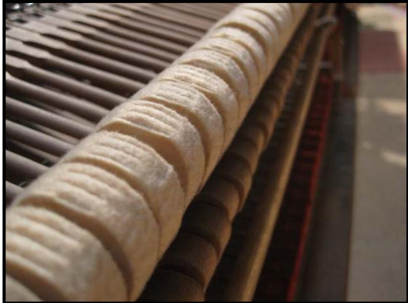
No matter how good the tuning of a piano, or to what extent other repair work has been done to a piano with a set of hammers in this condition, the resulting tone will be less than optimal.
